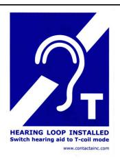
We have recently installed a system in the sanctuary called the "Hearing Loop System". This system works with hearing aids that have a "T-Coil" installed and sends sound directly to the hearing aid from the present sound system.
